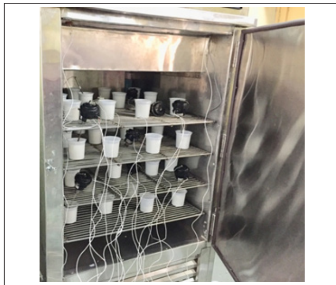
Figure 4: Sensing temperature of dahi by placing temperature sensors in dahi cups and the cooling fans placed on the top used for effective forced convection process
